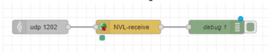
Figure 10: NVL receive flow in Node-RED
